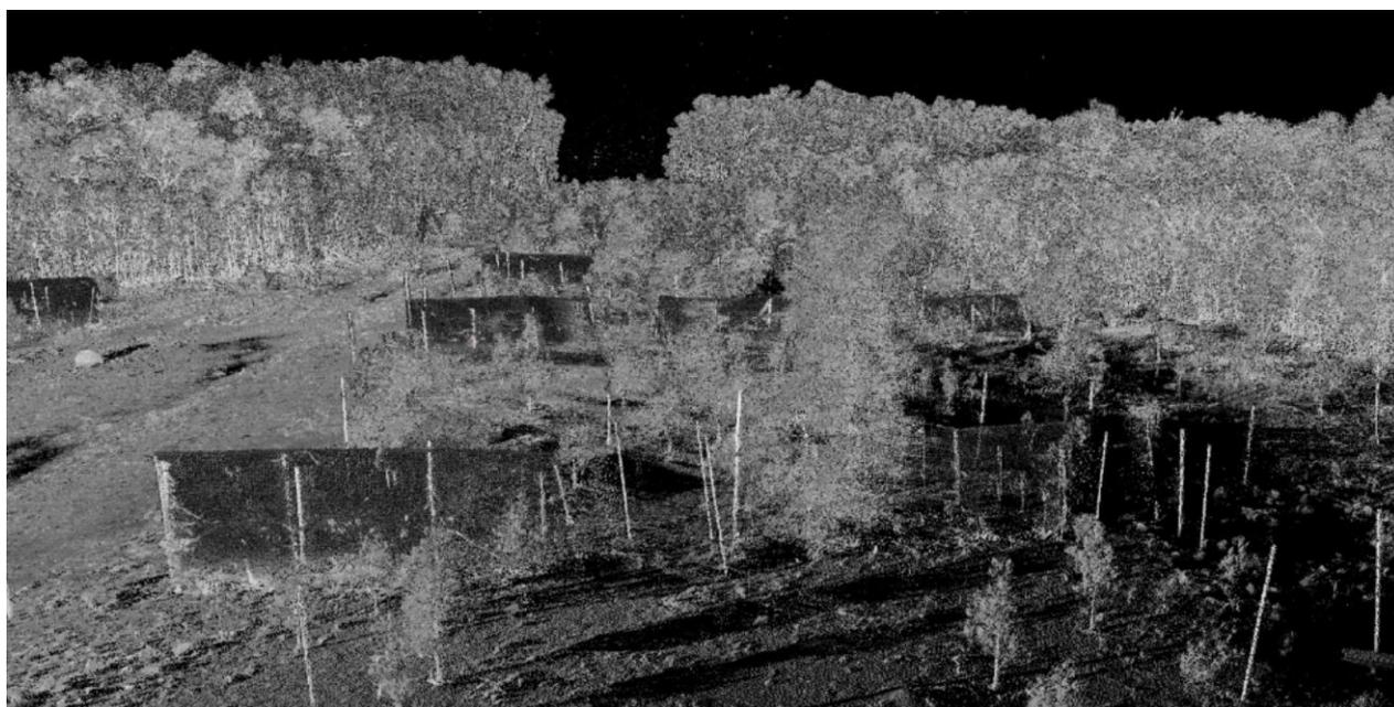
Figure 6 - Oblique reflectance view of the rehabilitation zone. Grayscale image shows the reflectance of the laser beam. The sky and wet soil show no reflectance (black) whereas the stems and leaves of mangroves show up in whiter shades. Recruitment fences are visible in the laser reflectance data with the support poles in white and the fencing mesh in darker shades.
