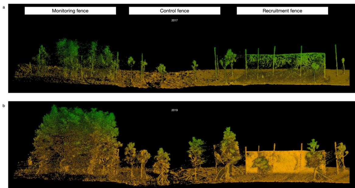
Figure 15 - Side view of terrestrial laser scanning data collected across a monitoring, control and recruitment fences in 2017 (a) and 2019 (b).
