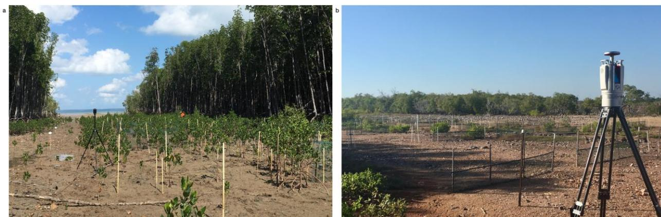
Figure 5 - Terrestrial laser scanning at the GEP rehabilitation site. a) Scanning with the light-weight Leica BLK360 in the tidal creek assemblage in 2017; and b) scanning with the long-range Riegl VZ-2000i in 2019 in the hinterland margin assemblage.
